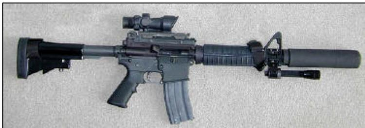
On a 5.56mm carbine, the BR T8 suppressor (left) reduces the noise of the shot by approximately 82%, making it only a few decibels louder than a .22 rimfire rifle. This design is perfect for use by high mobility entry and tactical teams or by sniper teams where rugged equipment is needed without maximum sound reduction. The Reflex suppressor is also the best choice for large calibre rifles because it
